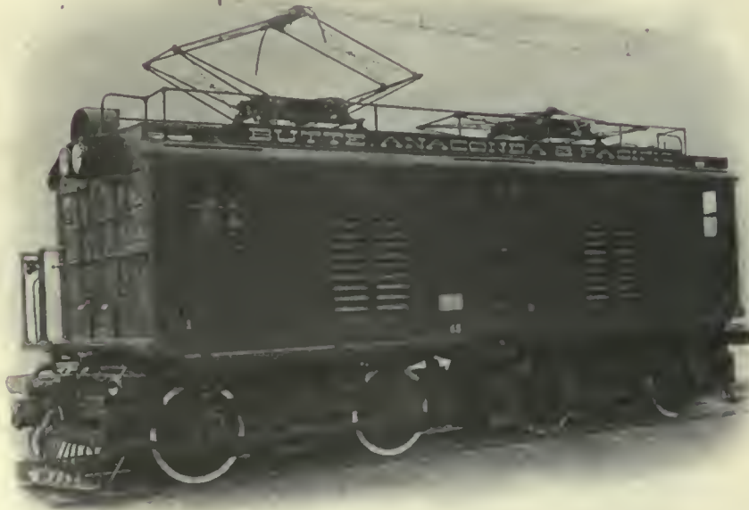
FIG. 536. ELECTRIC LOCOMOTIVES. Electric Locomotive for 2,400-Volt Direct Current Overhead Contact Operation, Butte, Anaconda & Pacific Railway.
